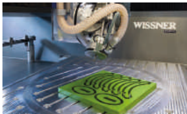
5D milling with rotating spindle and rotary table
