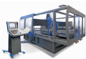
Rotary table, thus providing two autonomous work zones
